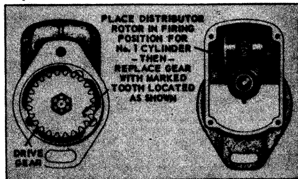
Fig. 2. DRIVE GEAR MARKING AND ASSEMBLY
